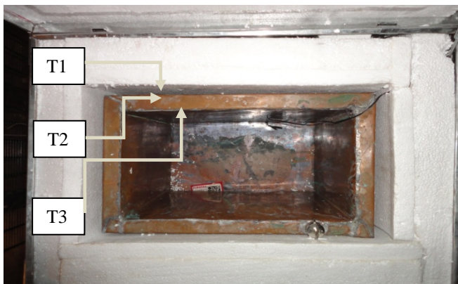
Fig. 5 (T1, T2, T3 section of Thermal Reservoir)
